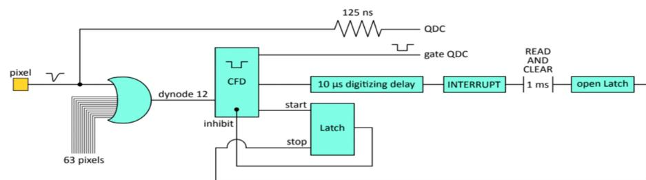
Fig.1 Diagram showing data-acquisition system. Analog signals from each pixel were passed to VME QDCs and OR'd onboard the H12700 MAPMT. The OR'd signal was then used to trigger the DAQ
