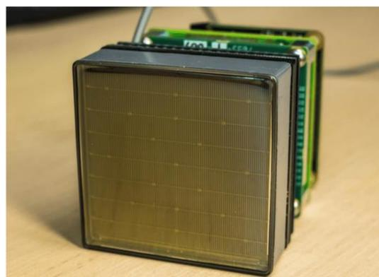
Fig.3 Hamamatsu H12700 MAPMT with GS20 lithium glass scintillator mounted using silicon rubber.
