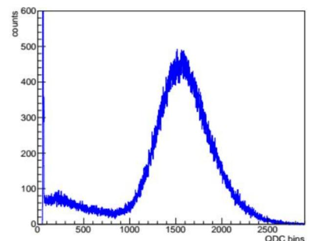
Fig.6 Response of the non-pixelated neutron detector to the uniform mixed gamma-ray and neutron fields presented by the Am/Be source. The sharp peak located at channel 50 corresponds to the QDC pedestal. The broad peak centred at channel 1550 corresponds to neutrons.
