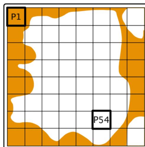
Fig.5 Map of air bubble (white) on face of MAPMT contrasted against the region of ideal optical contact (orange), caused by silicone elastomer.
