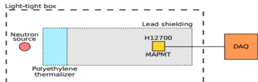
Fig.2 Schematic overview of light tight box. From the left: neutron source, layer of thermalising polyethylene, and lead castle containing the pixelated detector
