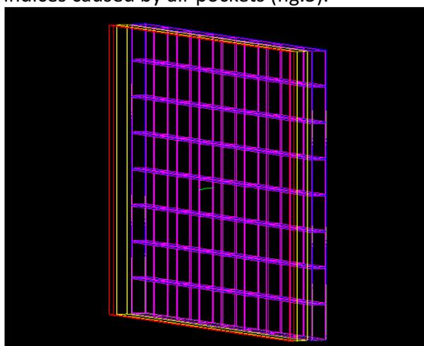
Fig. 4 Monte Carlo simulation performed using Geant4 software. The red structure indicates the GS20 <sup>6</sup>Li scintillator glass, the yellow structure represents the optical window of the MAPMT, and the purple structure represents the pixelated photocathode. The small green line represents an incident optical photon.
